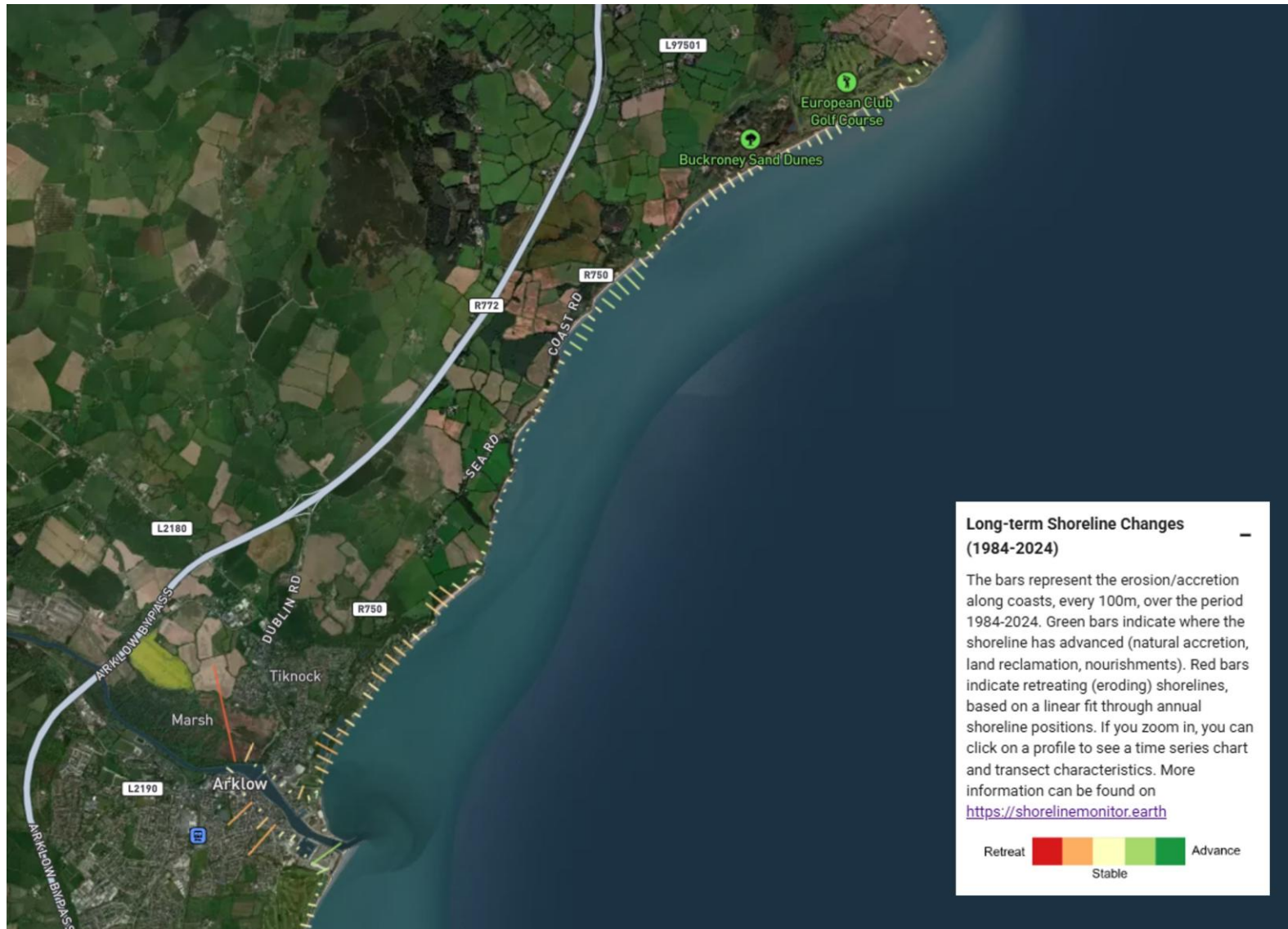
Figure 6.14: Shoreline change along the Wicklow Coast, with bars representing erosion/accretion at every 100 m over the period 1984 – 2024 (Luijendijk et al. , 2018).
